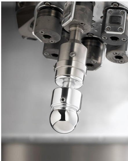
Fig. 6: The holder is set at an angle; each workpiece rotates independently.
