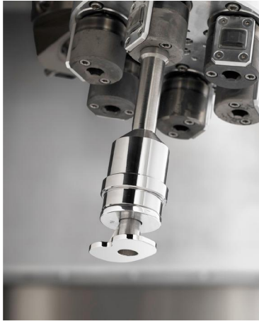
Fig. 7: Angled, independently rotating workpiece holder with tibia
