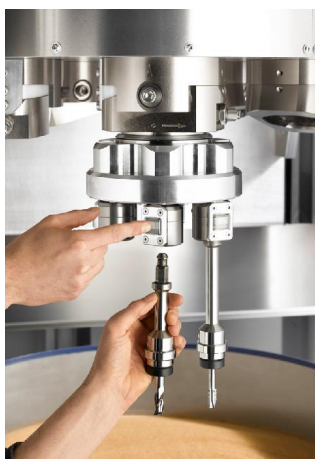
Fig. 5: Changing the workpiece in the independently rotating holder
