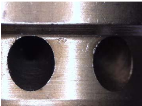
Picture 1 the burr is visible
