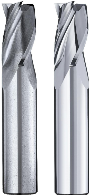
Figure 5: Tungsten carbide end mill before and after drag finishing
